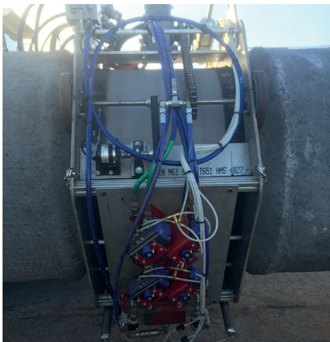
Figure 1. This automated liquid coating system reaps environmental benefits with an overspray recovery box that captures approximately 95 - 99% of fugitive emissions.
